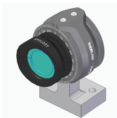
Figure 2.3: CAD model of the new optical isolator used for both lasers.
