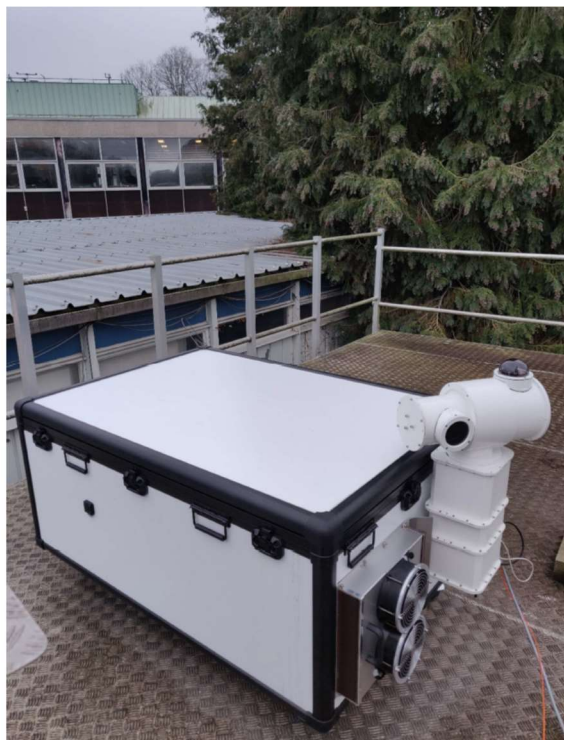
Figure: Enclosure box and solar tracker
