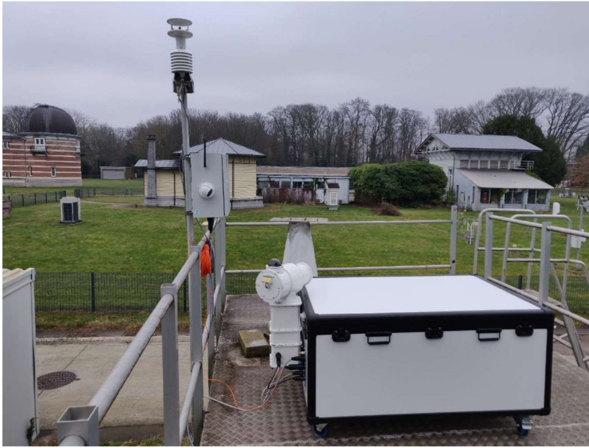
Figure: Enclosure box and meteorological station deployed for testing at the campus of BIRA
