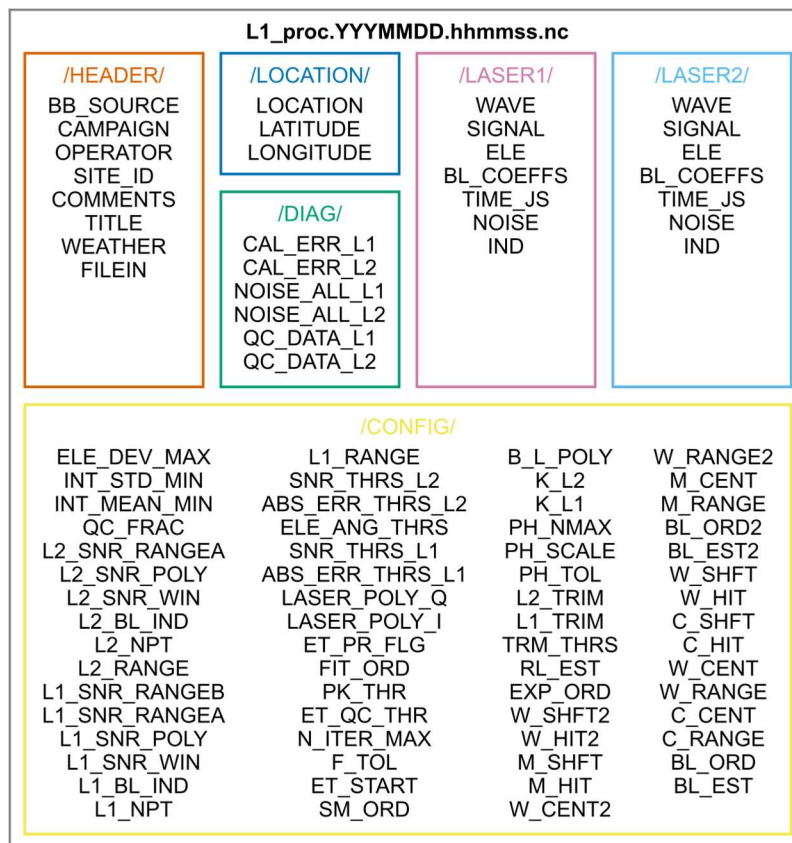
Fig. 5.7: Diagram showing the structure of the pre-processed L1 NetCDF file. Coloured boxes indicate a group. There are no global variables.
