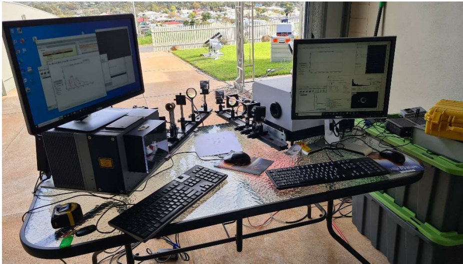
Figure 6. a. Two EM27/SUNs (left) and two Ekotrackers as deployed at Broken Hill. The fibre optic cables lead from the Ekotrackers to the two FTSs housed in the garage behind the green roller door (Figure 1b).
